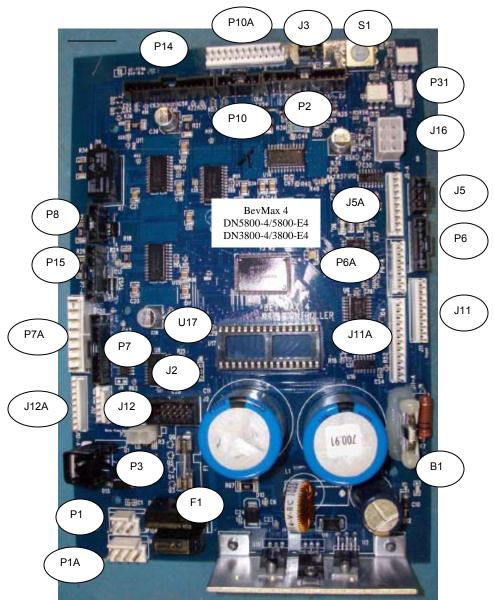
BEVMAX 4 DN5800-4/3800-4/5800-E4/3800-E4 MDB/EXE CONTROLLER CONNECTIONS
