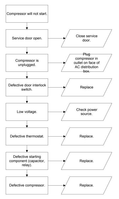
Troubleshooting Tip: Use a short 15 Amp extension cord and plug the compressor directly into the wall outlet. This will bypass the AC distribution box. Note: For Testing Purposes Only.
