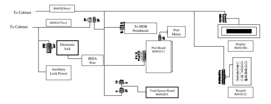
BevMax 4 Wiring Diagrams Pg 2 of 3 803,889,16x.x1 Exp. Fluor. 803,889,53x.x1 Exp. LED 803,889,52x.x1 Dom. LED 803,888,47x.x1 Dom. Fluor.
