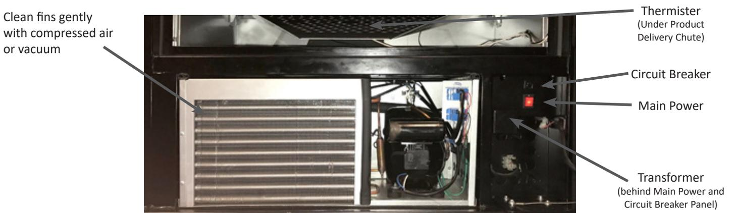
**WARNING THE COMPRESSOR ELECTRICAL CIRCUIT IS ALWAYS LIVE WHEN THE PLUG IS CONNECTED TO AN ELECTRICAL OUTLET. FOLLOW PROPER SAFETY PRECAUTIONS WHEN CLEANING THIS AREA.**
