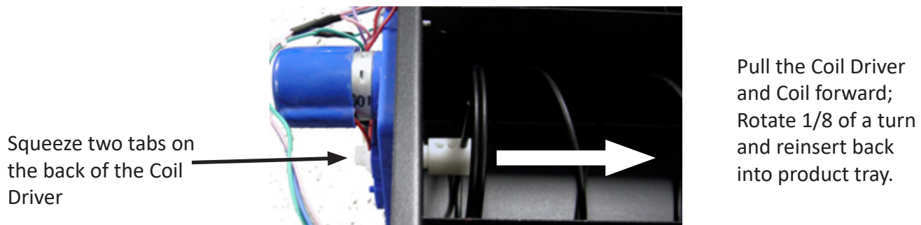
Figure 10 – Coil Rotation Adjustment
